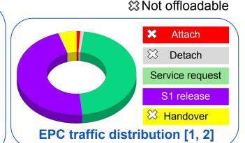
TurboEPC offloads *S1 release* & *Service request* messages to the programmable switch at the edge
