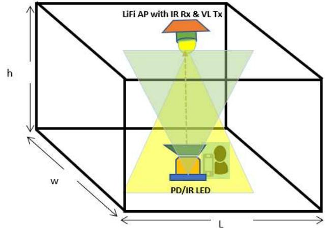
**Fig. 1.** Uplink and downlink indoor LiFi network communication model.
