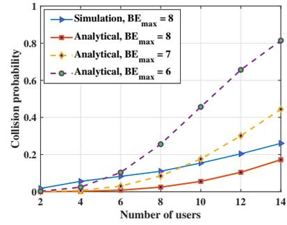
**Fig. 5.** Average network collision probability analysis for different backoff values using HCCA uplink MAC protocol in LiFi network.
