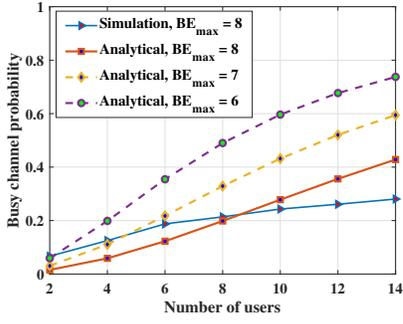
**Fig. 7.** Average network busy channel probability analysis for different backoff values using HCCA uplink MAC protocol in LiFi network.
