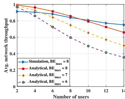
**Fig. 3.** Average network throughput for different  $BE_{max}$  value using HCCA uplink MAC protocol in LiFi network.
