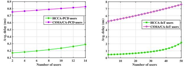
**Fig. 9.** Average delay for PCD and IoT users respectively using CSMA/CA and HCCA uplink MAC protocol in LiFi network.
