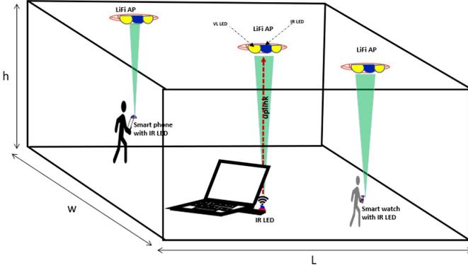
**Fig. 2.** Illustration of uplink communication using IR LED in LiFi network for different types of gadgets carried by the user.
