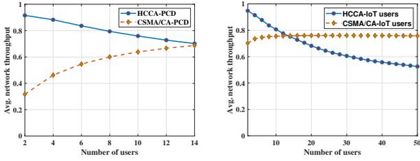
**Fig. 4.** Average network throughput analysis for PCD and IoT users using CSMA/CA and HCCA uplink MAC protocol respectively in LiFi network.
