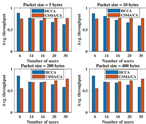
**Fig. 12.** Choosing MAC protocol based on average throughput, packet size, and the number of users using hybrid MAC mechanism.
