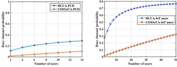
**Fig. 8.** Average network busy channel probability for PCD and IoT users respectively using CSMA/CA and HCCA uplink MAC protocol in LiFi network.
