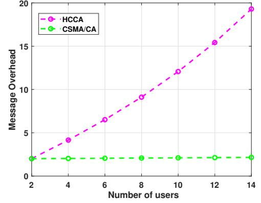
**Fig. 11.** Comparison of message overhead for HCCA and CSMA/CA MAC mechanisms.
